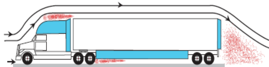
B: A tractor-trailer with aerodynamic devices installed produces less drag (shown as shaded area)
