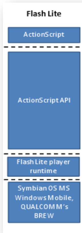
Figure 2.3: Flash Lite Framework Stack
