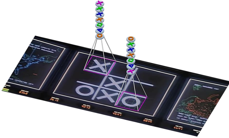
Figure 14: Hypercolumns of neurons in a convolutional layer [5 \times 5 \sim 3 | 3 \rightarrow h] showing different types of neurons. There are 7 neurons mapped in the same spatial region of the input image, which correspond to an output hyperdepth h = 7 of the convolutional layer.
