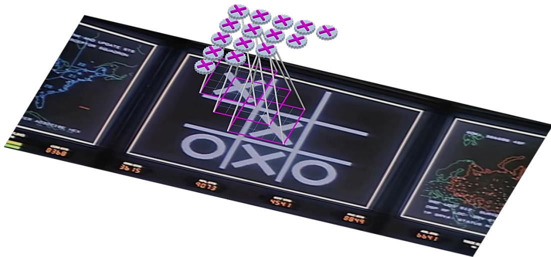
Figure 13: Spatial arrangement of overlapping neurons in a convolutional layer [5 \times 5 \sim 2 | 3 \rightarrow h] . All neurons for the magenta-colored X-shaped feature, share a common slice of weights of the 4D convolutional kernel. (Input sample is a frame from the 1983 MGM movie “War Games” depicting an AI trying to find a winner in Tic-Tac-Toe).
