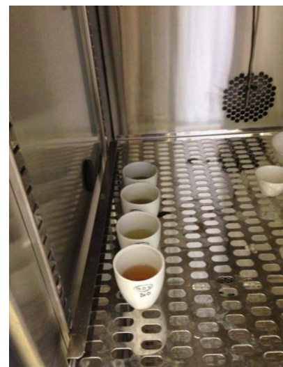
The samples in the oven at 60 degrees
