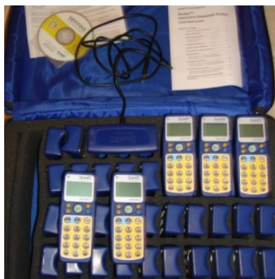
Εικόνα 2.7 - Senteo Interactive Classroom Response System- Receiver and 32 Student Clickers
