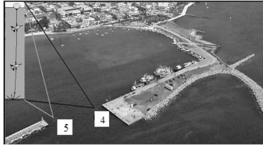
Fig. 3. Photo with a panoramic view of the harbour and a sketch of the deployment and location of the current meters at the entrance of the harbour
