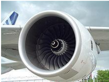
A Rolls-Royce Trent 900 engine on the wing of an Airbus A380
